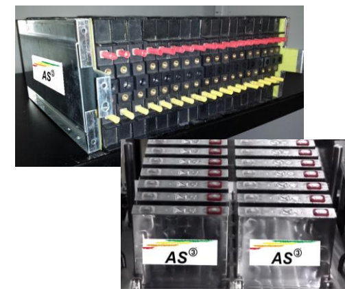
Battery Module Rack (4000Wh)
