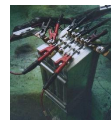
Court-circuit Short circuit
